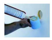
Press the MTH CILINDRO mounting cylinder into the milled hole in the insulation panel until it is flush. The blue colour provides for easy checking of all the MTH CILINDRO mounting cylinders.
